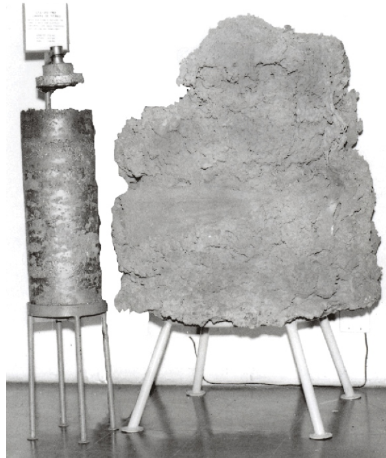
Figure 5: Titanium sponge (750kg) and titanium ingot (260kg) produced in CTA (Henriques, 2008).
