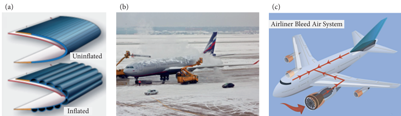
Figure 14. (a) Inflatable rubber boot method, (b) chemical spray method, and (c) bleed air method (Xie et al. 2016; Cao et al. 2015; Stothers 2013).
