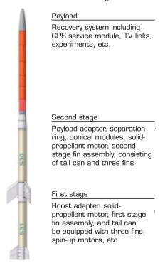
Figure 2. Schematic decomposition of a sounding rocket vehicle. Adapted from Garcia et al. (2011).
