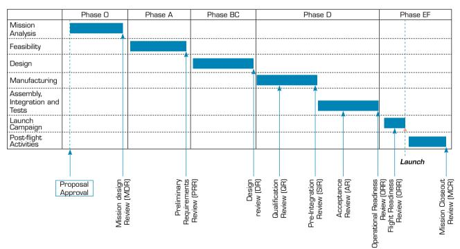
**Figure 4.** Proposed life-cycle for sounding rocket missions from the BMP program.
