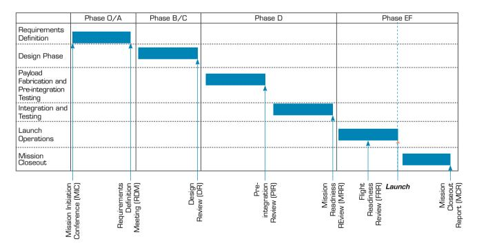
**Figure 8.** Life-cycle for sounding rocket missions from the NSRP program, as inferred from the mission schedule given in Fig. 7.
