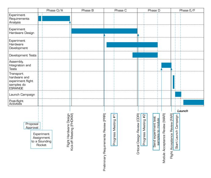
**Figure 6.** Life-cycle for sounding rocket missions from the ESA ELIPS program, as inferred from the mission schedule given in Fig. 5.
