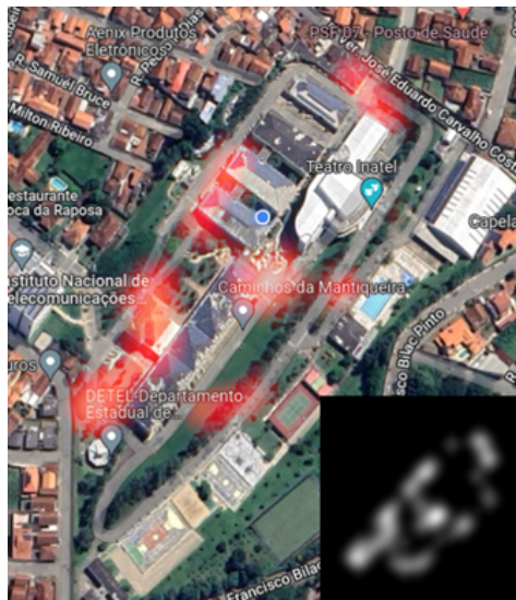
Figure 15. Natural gamma radiation levels read by the SEN-14209 module in different locations of the Inatel campus.
