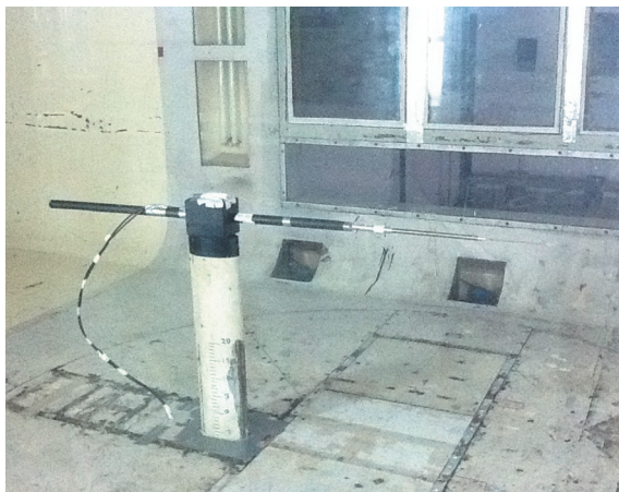
Figure 4. Hot-wire probe in the TA-2 test section.
