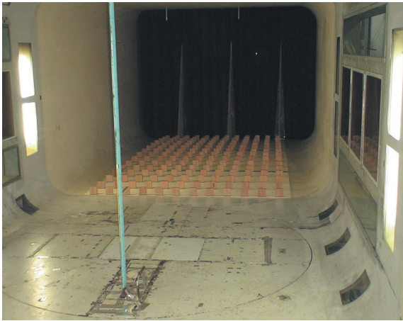
Figure 10. Configuration III – spires and roughness elements.
