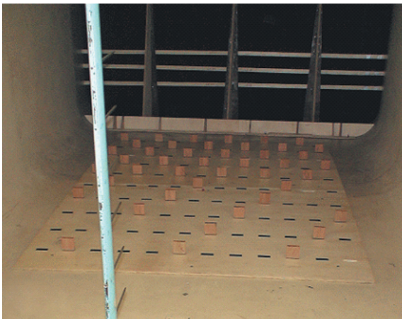
Figure 20. Configuration VIII – barrier, roughness elements, and strips. Measurement close to the mobile integration tower site.
