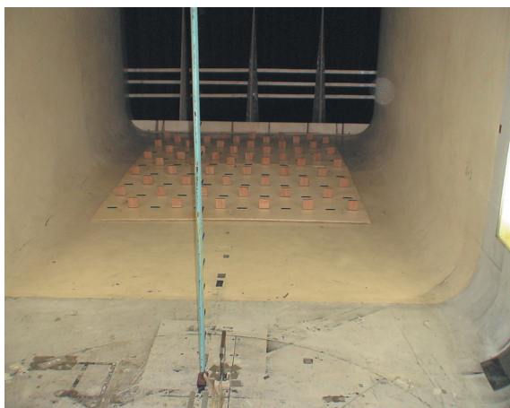
Figure 14. Configuration V – barrier and roughness elements.
