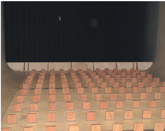
Figure 6. Configuration I – barrier and roughness elements.
