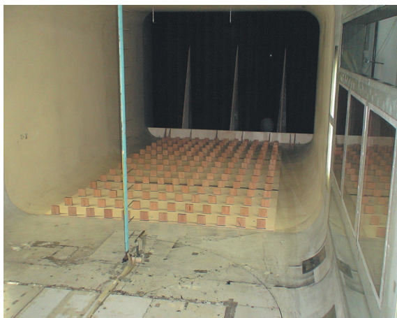
Figure 12. Configuration IV – spires, barrier, and roughness elements.
