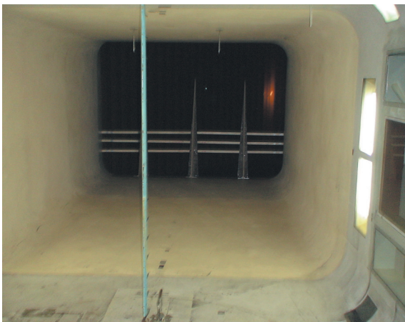
Figure 8. Configuration II – spires and horizontal strips.
