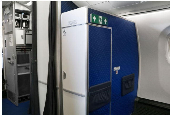
Figure 4. Embraer's wheelchair storage system.
