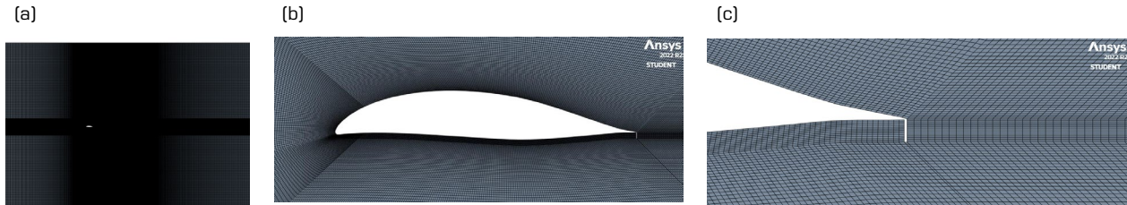
Figure 6. Numerical grid. (a) 2D airfoil in a rectangular grid; (b) meshing in the vicinity of the airfoil; (c) close-up mesh around the GF.
