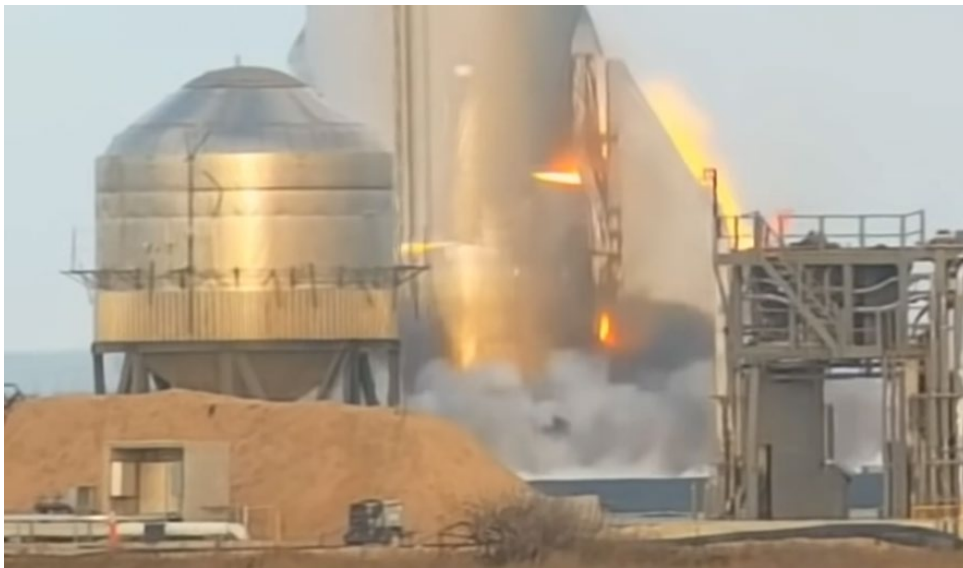
Figure 8. Onset of the explosion in the main oxygen tank's lower region.
