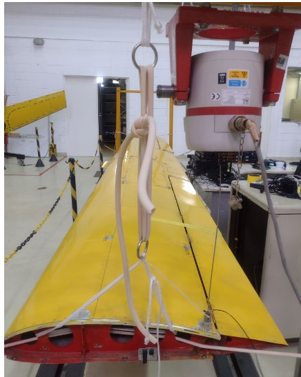
Figure 9. Shaker/stinger/force transducer fixed to the wing structure.
