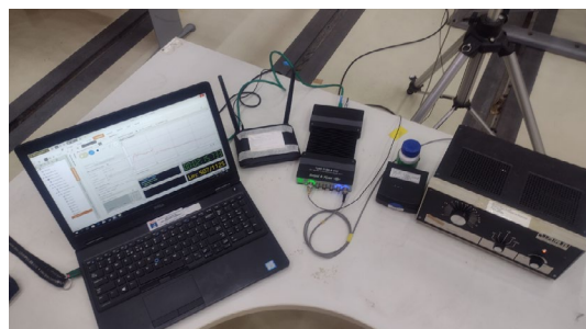
Figure 4. First experiment structure displayed. A Brüel & Kjaer DAQ Module Type 3160-A-042 connected to a low-cost COTS Wi-Fi router.
