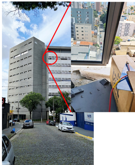
Figure 11. Outdoor test with the SDR using the directional LPDA, in detail, the antenna on the window ledge.
