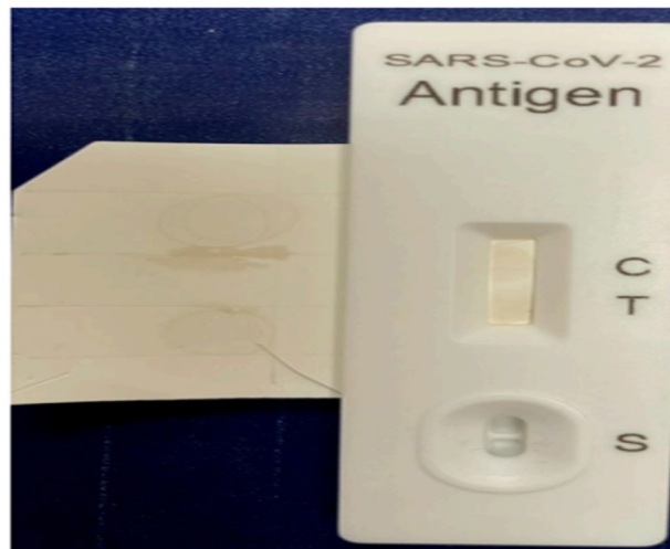
Figure 2. Photo of the housing used in this method to demonstrate how compressing the lateral flow strip improves reliability. The actual size of the device is comparable to the SARS-CoV-2 detection kits.
