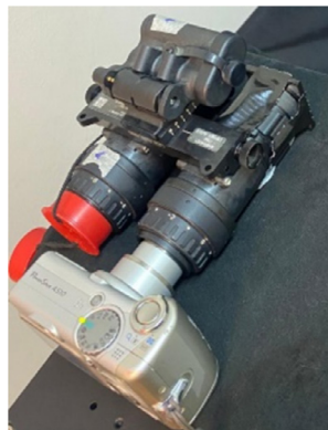
Figure 1. NVG system used in the standard optical setup. The gray device is the Canon PowerShot A510 camera, and the black device is a Generation 3 NVG.
