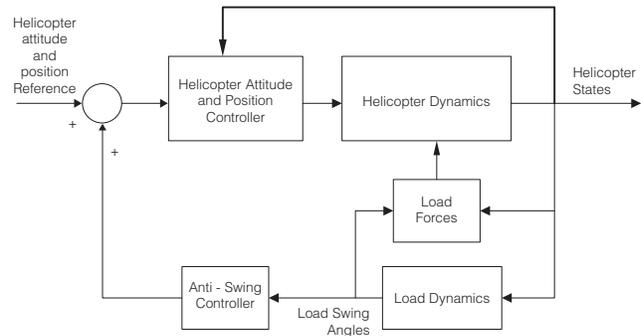
Figure 3. Configuration of the proposed anti-swing controller.
