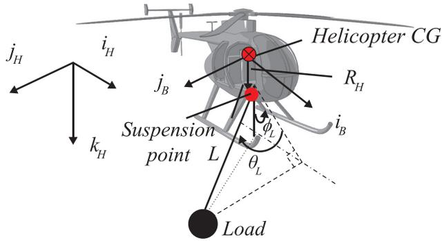
Figure 1. Configuration of helicopter with a slung load.
