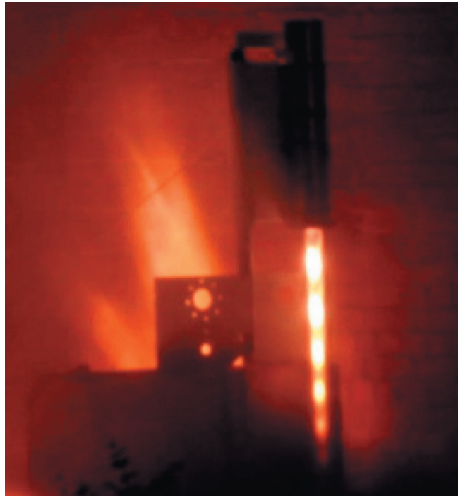
Figure 18. A paraffin/N 2 O hybrid rocket firing test at the University of Brasília.
