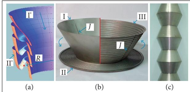
**Figure 1.** Graphic representation of the mathematical model for: (a) Fragment transformation of the initial conical shell (I') into a single corrugation (II'); (b) The transformation stages of the metal TVS shell; (c) Design solution for multi-conical TVS. J represents the welded joints of the shells.
