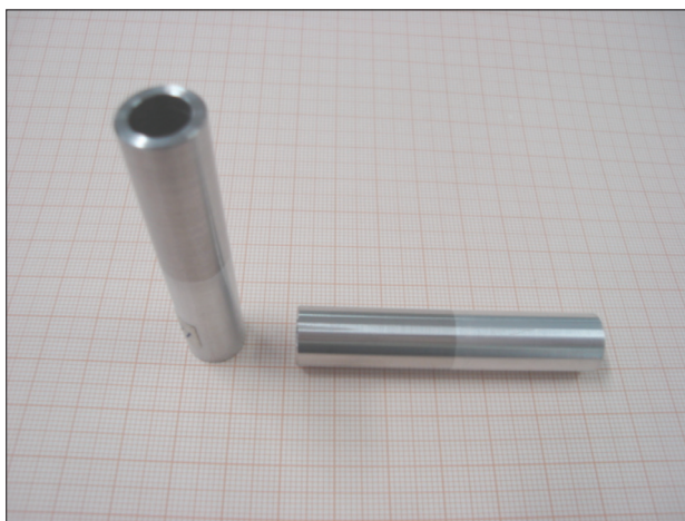
Figure 11: Joints produced by the rotary friction welding process (RFW) (dark part: AISI 304 stainless steel; clear part: AA1050 aluminum).
