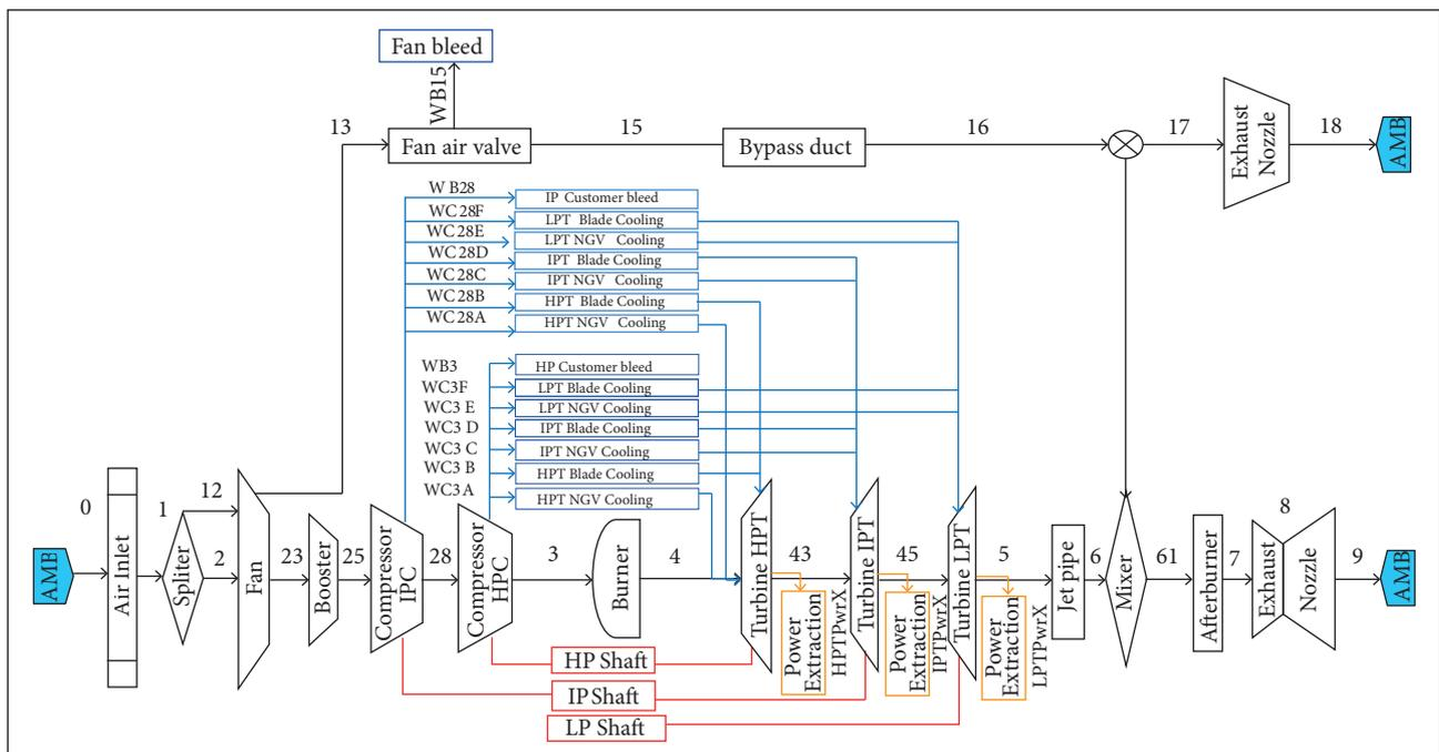
**Figure 1.** Three shaft direct drive engine model diagram.
