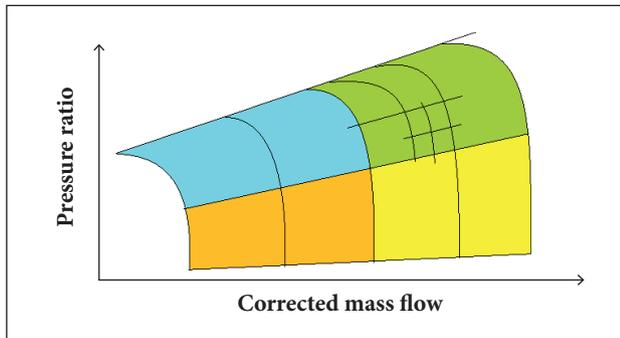
**Figure 4.** Quadrant division example in a compressor map.
