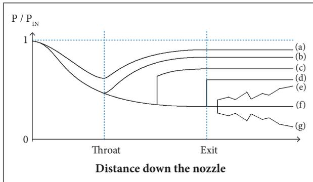
**Figure 3.** Pressure distribution through the nozzle (Devenport 2001). (a) Not choked at throat; (b) Just choked at throat; (c) Shock in nozzle; (d) Shock at exit; (e) Overexpanded; (f) Design condition; (g) Underexpanded.
