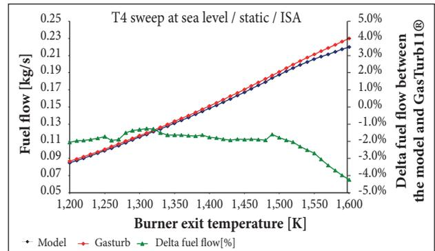
Figure 9. Two shaft simulated engine fuel flow comparison.
