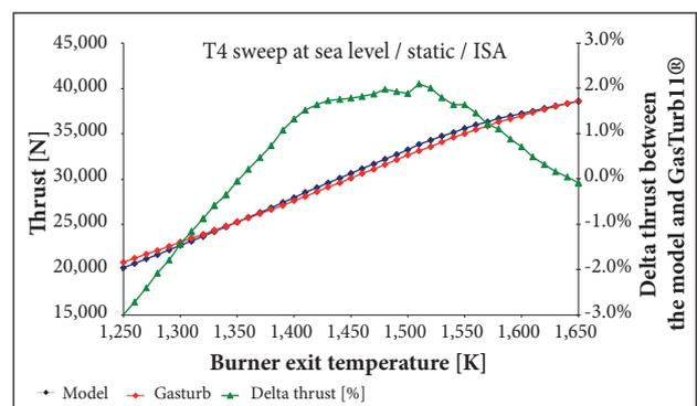
Figure 10. Three shaft simulated engine thrust comparison.
