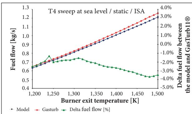
Figure 7. Single shaft simulated engine fuel flow comparison.
