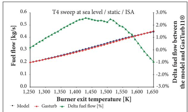
Figure 11. Three shaft simulated engine fuel flow comparison.
