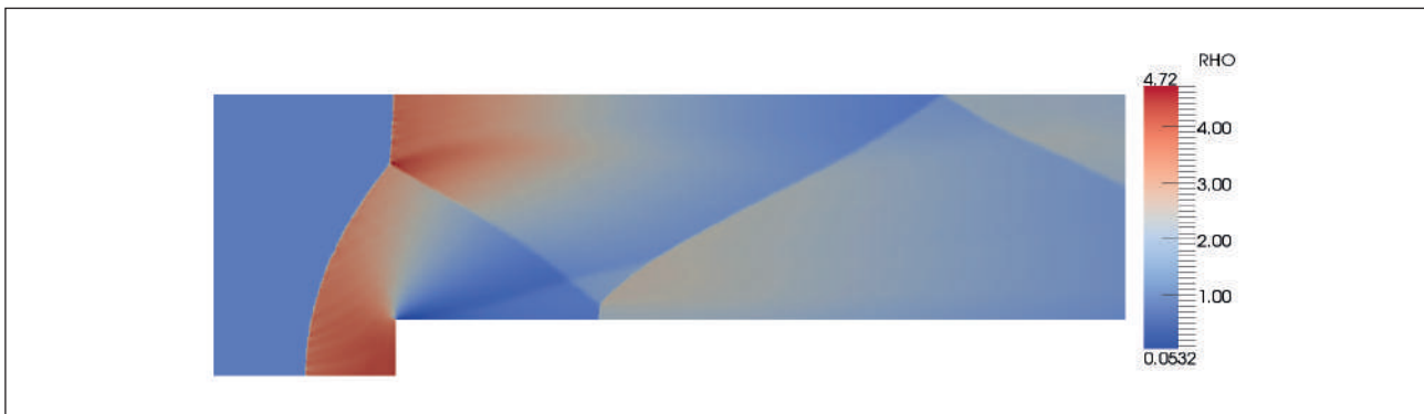
Figure 27. Density contours at the CV mesh level for the 3rd-order SFV method.
