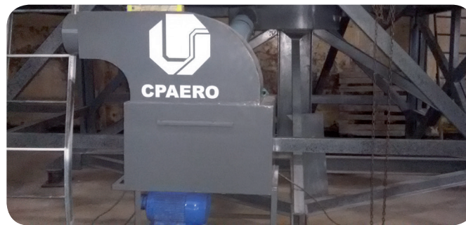
Figure 28. Cooling system to extract hot air inside the engine cavity.
