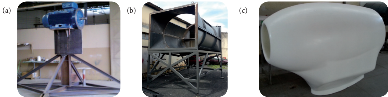
Figure 27. (a) Engine support; (b) Drive system section; (c) Engine fairing.
