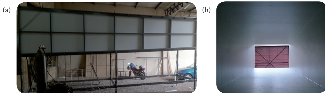
Figure 22. (a) Smaller diffuser; (b) Internal finishing details.
