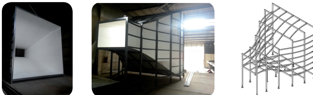
Figure 24. Contraction section (details of construction).
