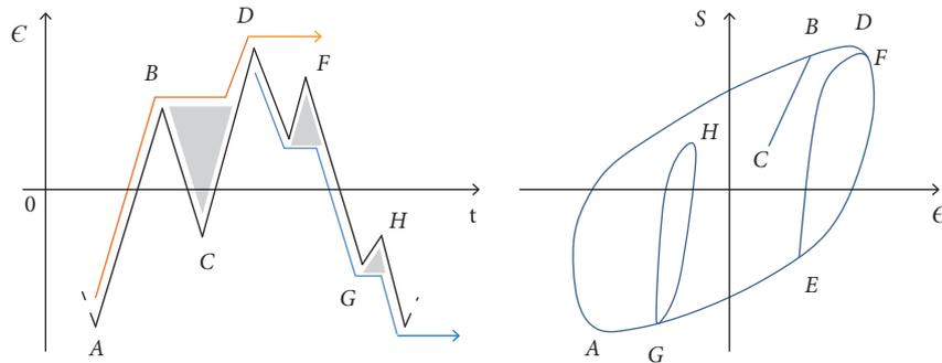
**Figure 4.** Stress-strain cycles. Adapted from Musallam and Johnson (2012).
