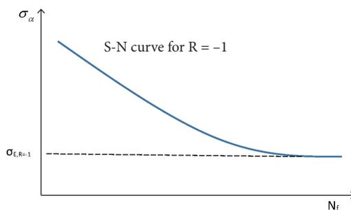
**Figure 5.** Schematic representation of an S-N curve.
