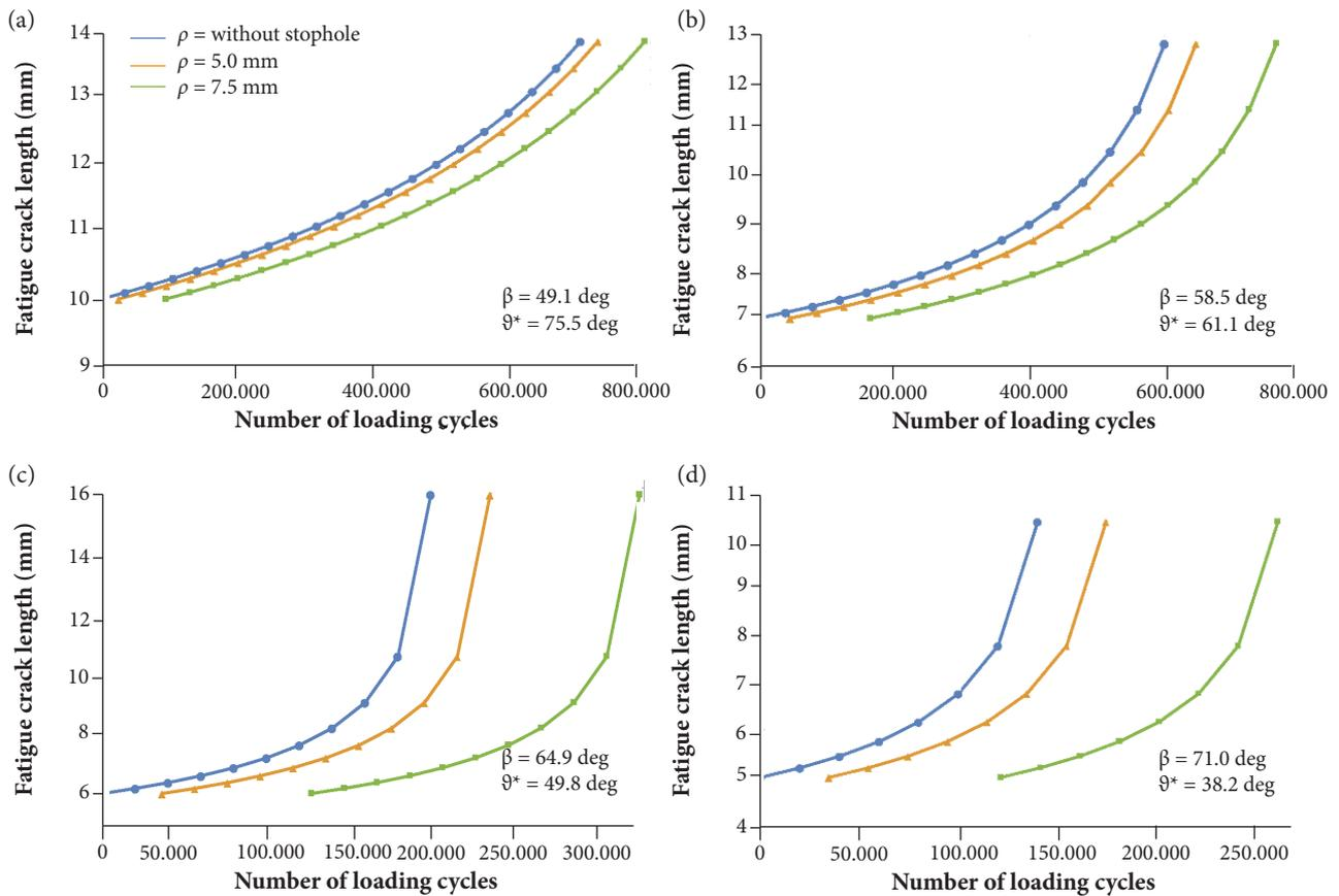
**Figure 9.** Crack length versus number of cycles for (a)  $\beta = 49.1$  deg., (b)  $\beta = 58.5$  deg., (c)  $\beta = 64.9$  deg., and (d)  $\beta = 71.0$  deg.
