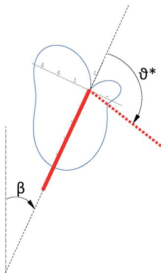
**Figure 3.** An inclined crack [with inclination angle  $\beta$ ] propagates in a direction  $\vartheta^*$  yielding minimum potential energy.
