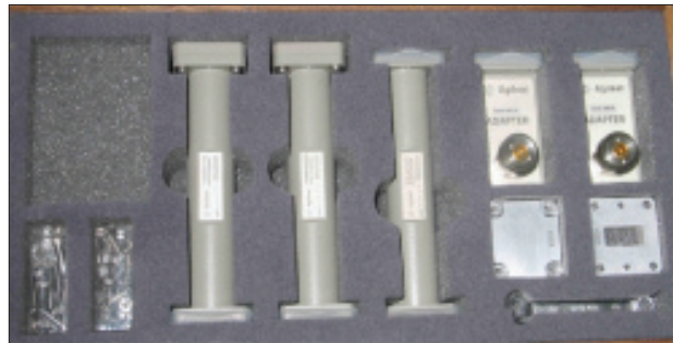
Figure 3: Waveguide calibration set for X band.
