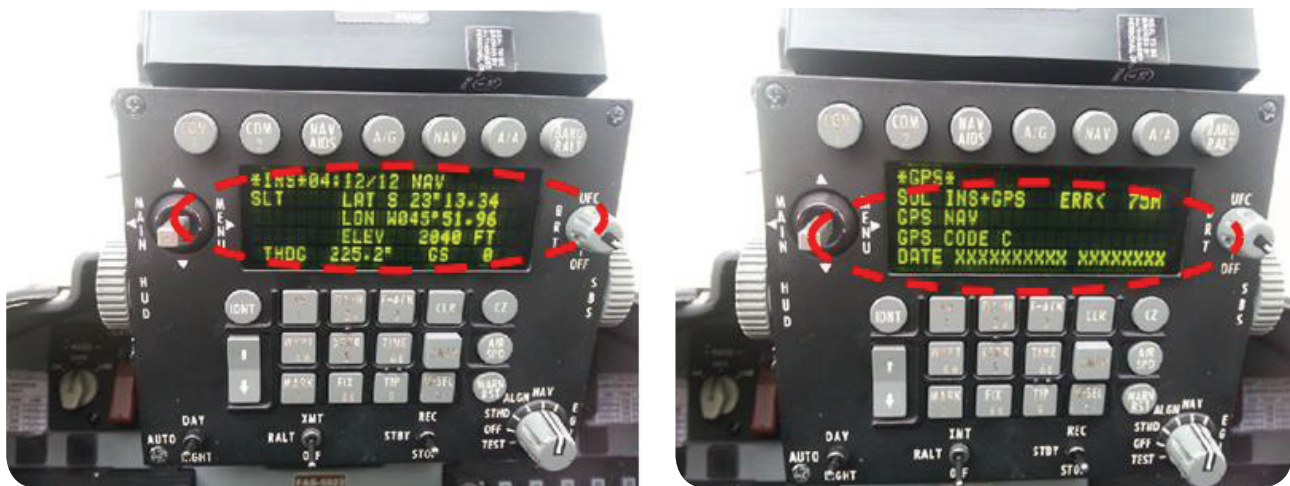
Figure 10. Aeronautical EGIR receiver under spoofing.
