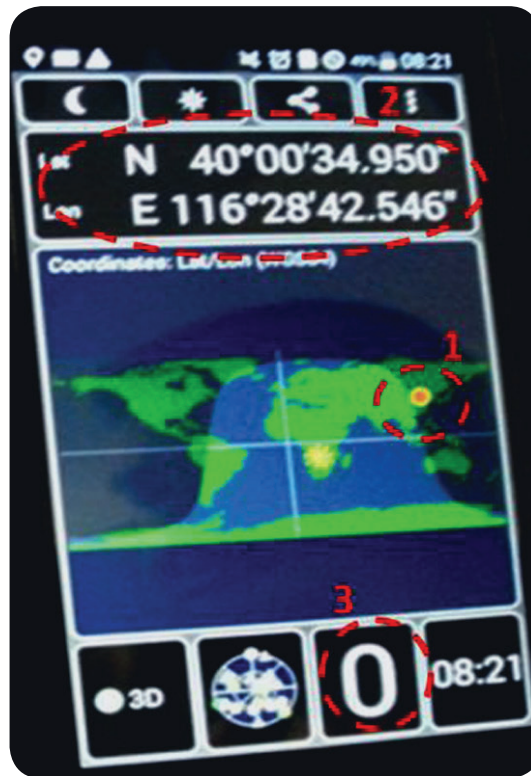
Figure 7. Mobile phone under static spoofing.
