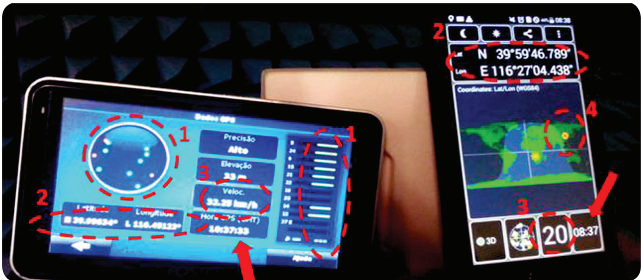
Figure 8. Automotive and mobile phone receivers under dynamic spoofing, with a date-time data close to the real ones.
