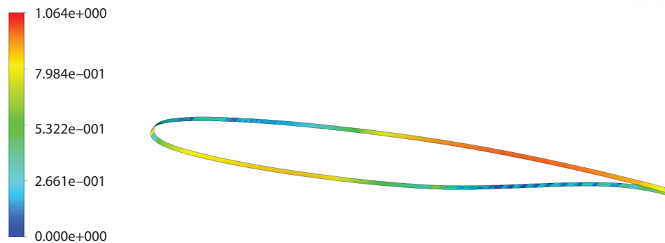
Figure 10. Y^+ calculated on the airfoil wall.
