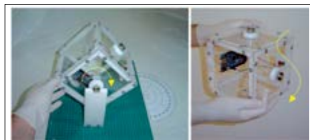
Figure 4. Two maneuvers of the CubeSat mockup for magnetometer data acquisition: rotation around one axis and aleatory motion.
