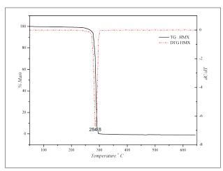
Figure 1: TG and DTG curves of HMX sample in atmosphere of N,
