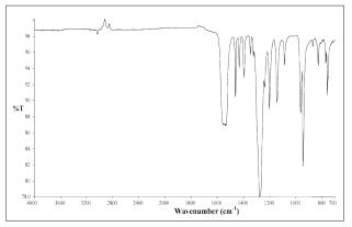
Figure 4: FT-IR/ATR spectrum in crystal germanium of HMX
