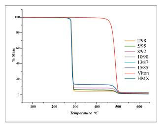
Figure 3: TG Curves of the system HMX/Viton sample in atmosphere of N,
