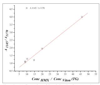
Figure 9: Medians values of the relative absorbance  $A_{1145} / A_{1170}$  as a function of HMX/Viton content obtained by TG.
