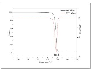
Figure 2: TG and DTG curves of Viton B sample in atmosphere of N<sub>2</sub>
